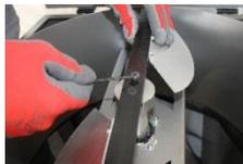
**2** Tighten the central screw of the shaft.
