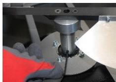
1 Loosen the lock screw shaft
