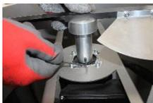
**1** Tighten the screw shaft blocker
